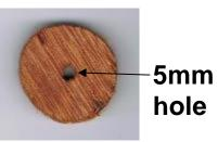
Rudder tube on hull floor disc (Ply).
