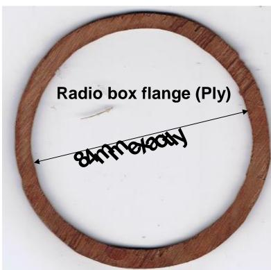
This ring is epoxied inside the deck over a an exact 84mm hole in the deck.
